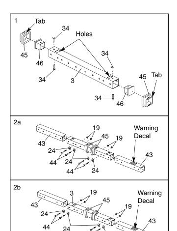
3. Note: The following drawings show the Crossbar (3) adjusted to the standard width.
